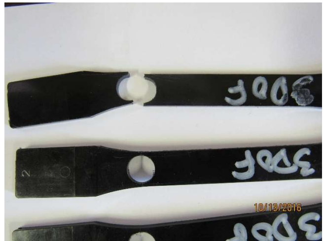
Figure 3: Broken 3 DoF parts.
